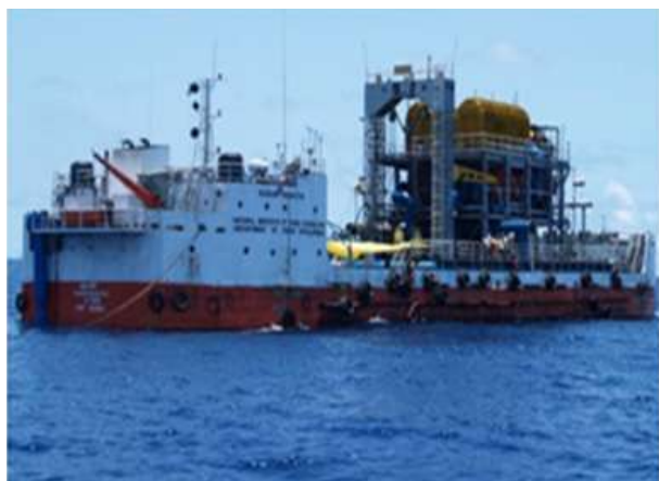
Barge mounted 1 MLD LTDD plant
