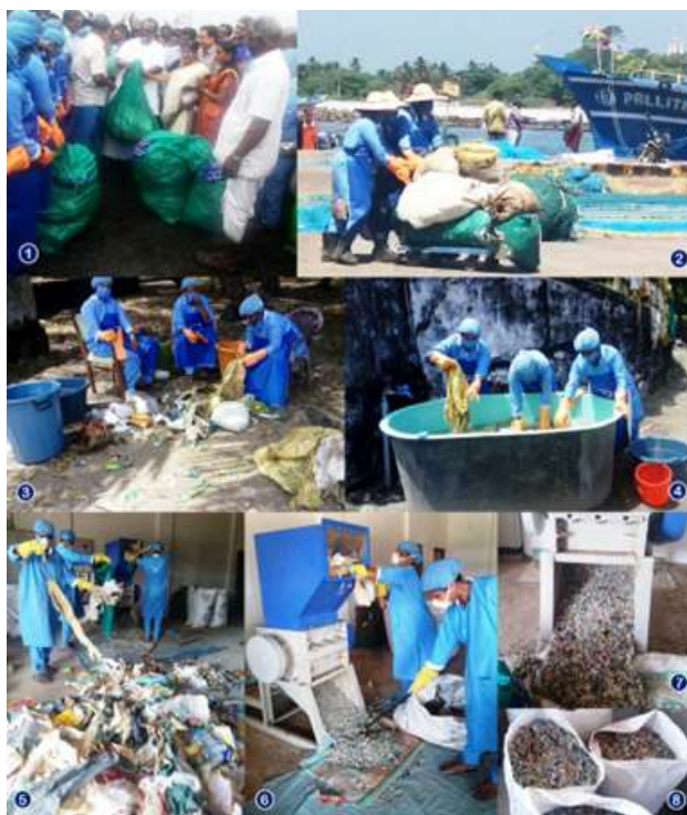
1. Receiving waste containing bags from boats; 2. Workers carrying the bags in trolleys to the segregation area; 3. Segregation of wastes; 4. Washing the plastic wastes; 5. Cleaned and dried wastes brought to the shredding unit; 6. Loading the plastic wastes into the shredding machine; 7. Shredded plastic product; 8. Stored in sacs for further use
